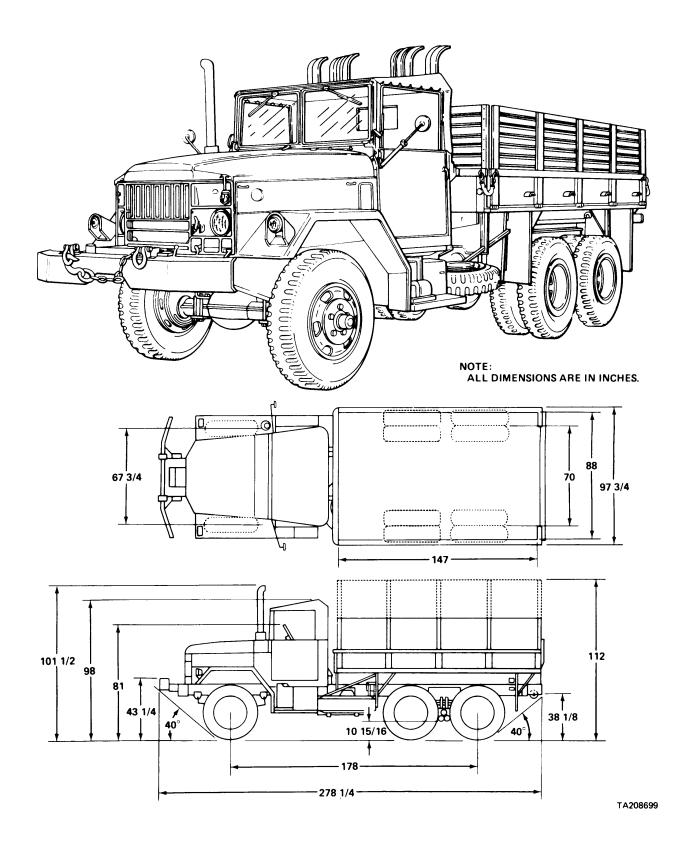
**PURPOSE**: This vehicle is employed by various support units primarily for cargo or personnel. It is especially well-suited for forklift cargo handling.
